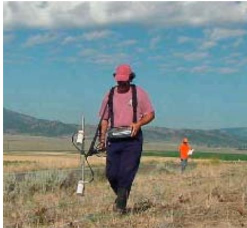
Figure 11.4. Cesium Vapor Gradiometer. Courtesy Billy A. Silva.
