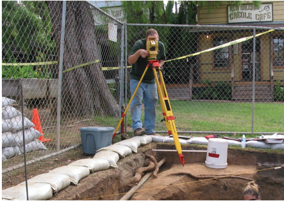
Figure 7.27a Scott Mattingly and Hillary Sweeney map the feature's profile with the total station. Courtesy Seth Mallios, David Caterino, and the South Coastal Information Center.
