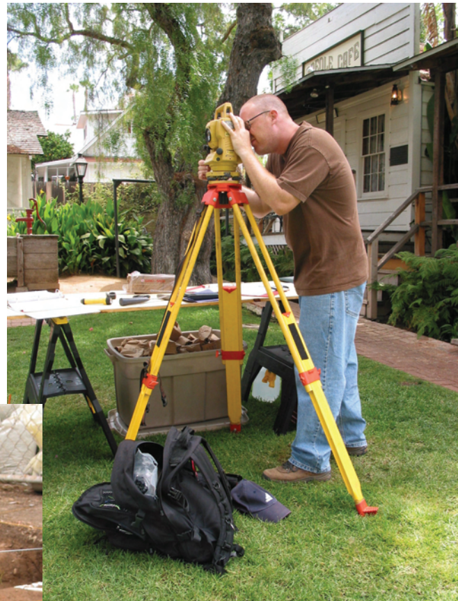
Figure 7.15 Scott Mattingly shoots in various data points using the laser transit. Courtesy Seth Mallios, David Caterino, and the South Coastal Information Center.
